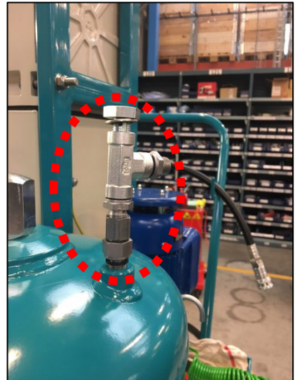
Figure 7: Example of inserting a T-connection on the air vent position to mount the hydraulic hose for the CMU outlet
