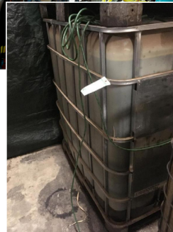
The waste oil from the washing process is placed in large totes for removal of water
