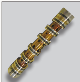
Varnish on valve spool
